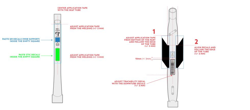
CENTER APPLICATION TAPE WITH THE SEAT TUBE PASTE EPAC DECAL 20MM BELLOW SEAT STAY WELDING (+/- 3MM)
