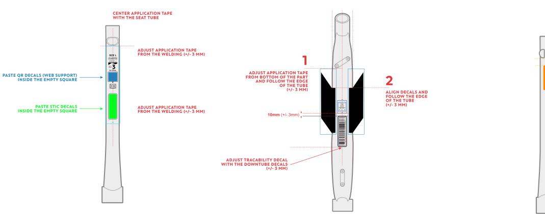
CENTER APPLICATION TAPE WITH THE SEAT TUBE PASTE EPAC DECAL 20MM BELLOW SEAT STAY WELDING (+/- 3MM)
