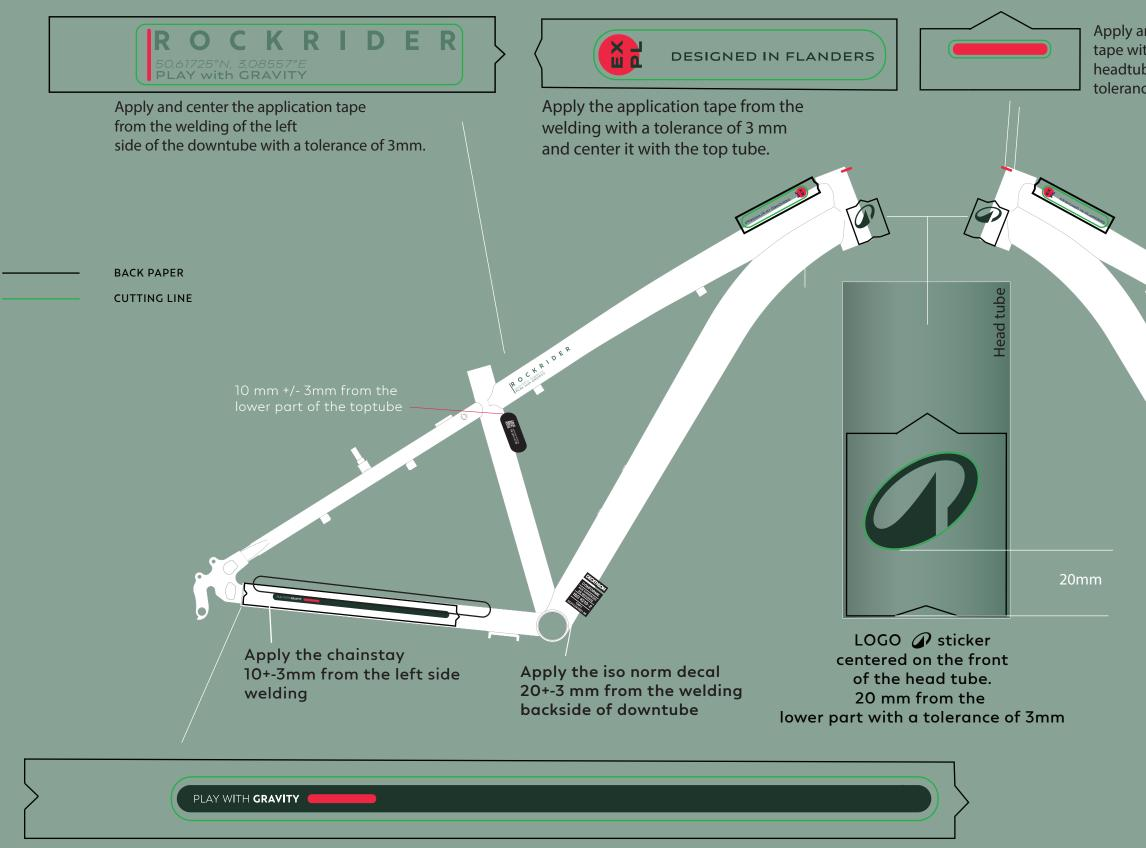
Apply and center the application tape on the right side of the chainstay tube from the left side welding with a tolerance of +- 3mm
