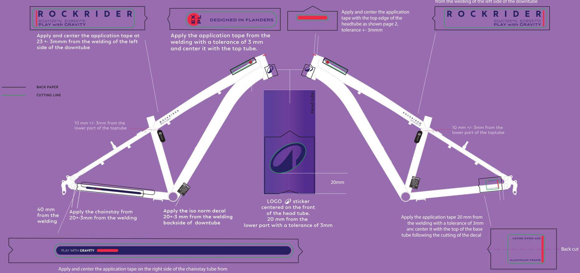
the left side welding with a tolerance of +- 3mm
