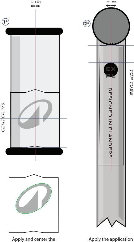
bottom part of the application tape with the down edge the headtube with a tolerance of 3 mm
